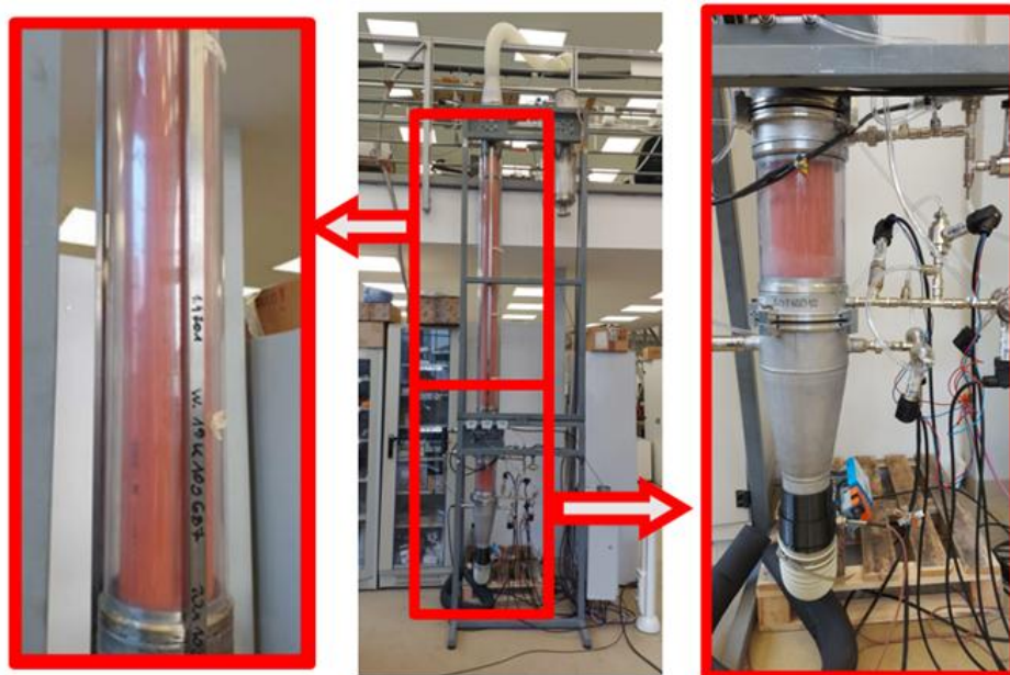
Figure 6. Experimental test stand with highlighted transparent polycarbonate pipe sections.
